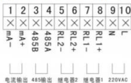
Wiring of 220VAC (four-wire system)
