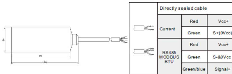
S=Signal, Vcc=Power Supply, GND=Vcc-&S-
